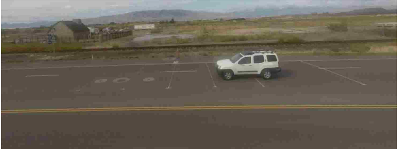
Figure 3-15: Image portraying painted lines used in LiDAR calibration (taken by a GoPro camera).
