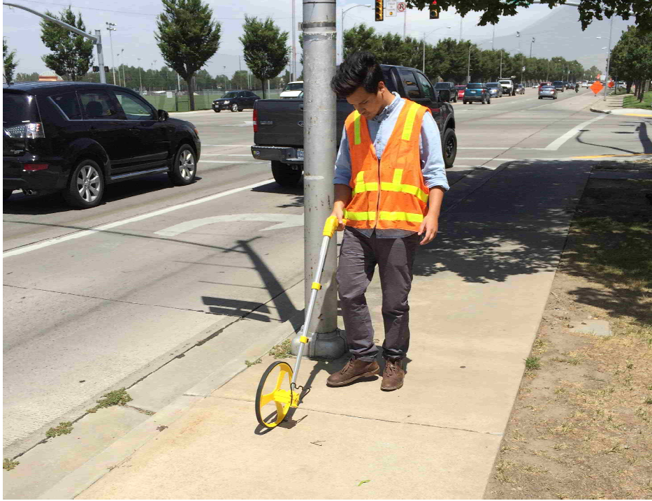
Figure 3-34: Measuring out the distance to place the cone (photo taken by Greg Sanchez).
